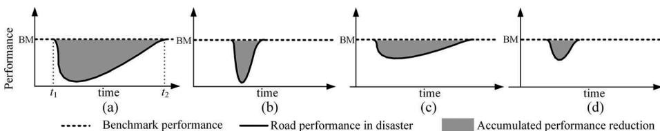
**Figure 1.** Possible scenarios of road network performance in a hazard. (a): a low-resilience scenario, (b-c): the intermediate resilience scenarios, (d): a high-resilience scenario.
